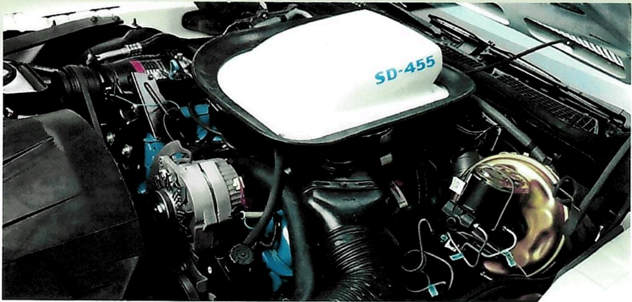
The SD-455 was the last salvo fired in the losing battle to keep muscle cars available to the public in 1973. It was a thinly disguised race engine with even a provision for a dry sump oiling system cast into the block. Pictured post restoration, this SD-455 remained with one owner for 40 years.
