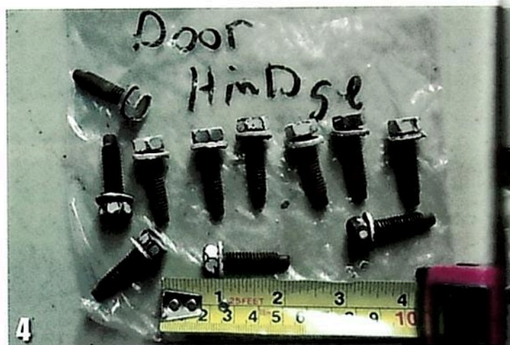
All of the hardware was bagged and labeled, then sent out to be reconditioned with the appropriate finish.
