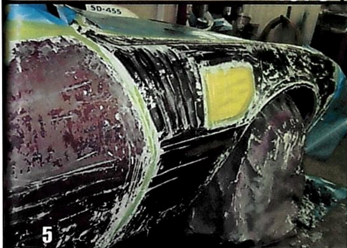
5 The Trans Am's body was stripped of its paint using chemical stripper. A one-owner Southern car, it was rusted in only a few of the typical spots.
