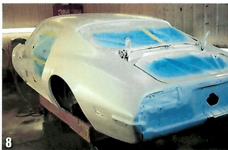
8 The body shell was primed and block sanded multiple times before it was ready to paint: about 480 labor hours from stripping to painting.
