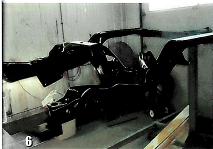
6 All of the chassis hard parts were media blasted, then finished with modern urethane primer and paint replicating the original colors.
